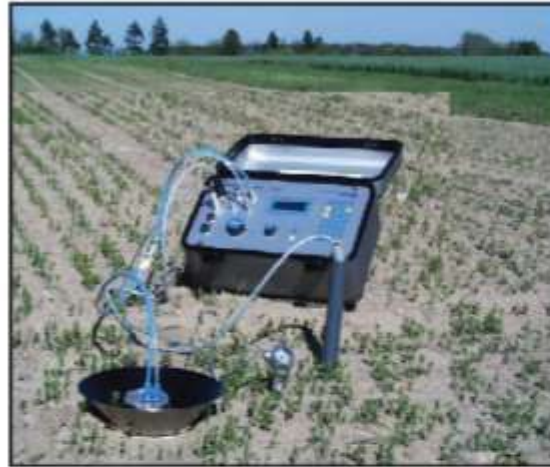
Air permeameter in the field measurement
